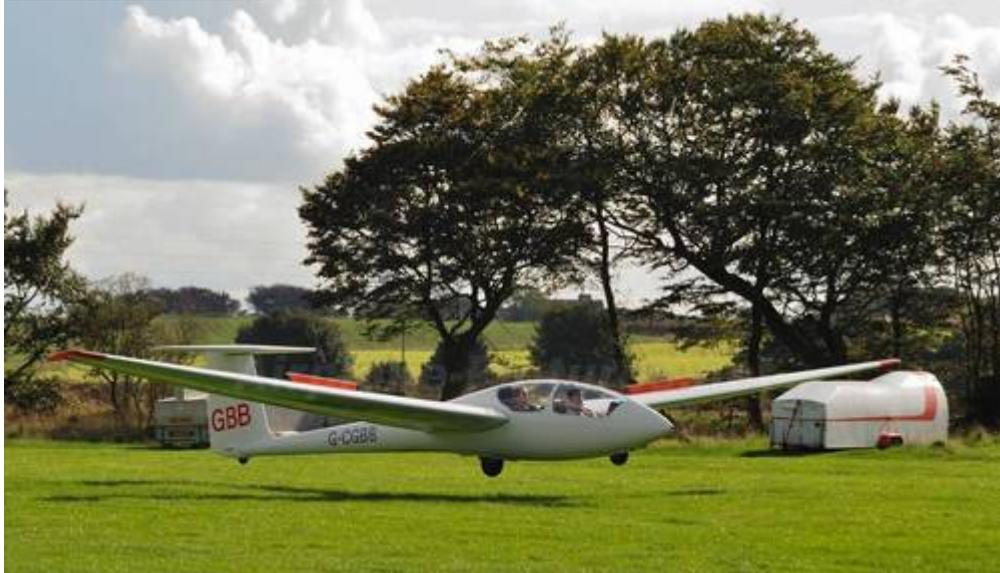
**Correct landing attitude.** Main & tail wheel will touch simultaneously. Nose held up.
