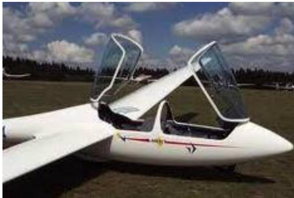
**Both canopies MUST BE CLOSED at all times**, except when getting in and out. Even walking a few feet away to hook up the ground or aero tow rope will leave the canopies exposed to damage.
