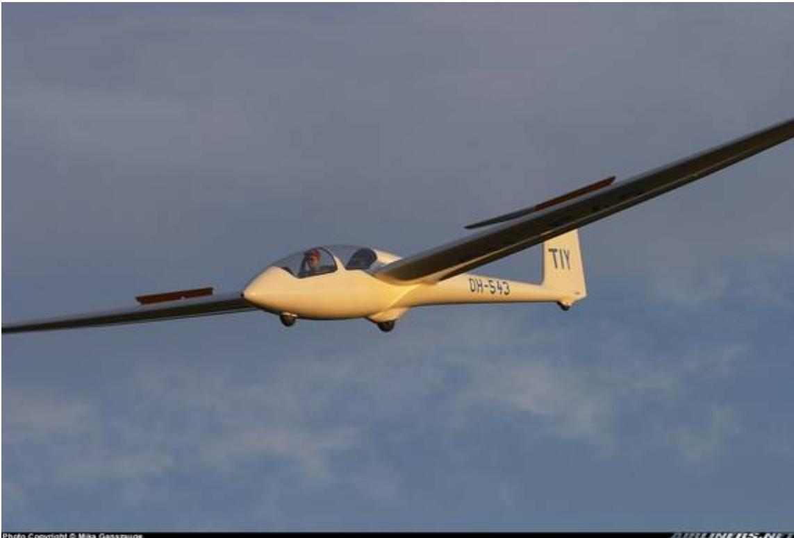
ASK-21 on final approach, before "roundout" or flare to land on main and tailwheel. Use about  $\frac{3}{4}$  Airbrake, 55 knots max. through the "mail slot" at the end of the runway.
